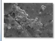
Biofilm formed on an TiAl6V4 implant surface S. epidermidis ATCC 35984
